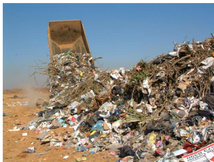
Figure 6 Building the intermediate windrow
