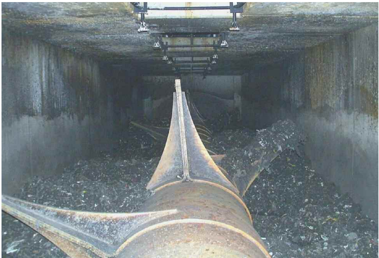
Figure 4 Inside View of a Percolator
