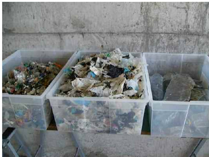
Figure 8 Plastics after shredding and washing (mixed plastics, polyethylene film and PET)
