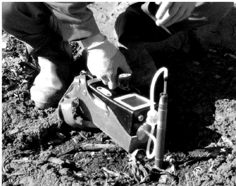
Photo 1 : CH 4 and CO 2 measurements on soil gas (Ecoprobe 5)
