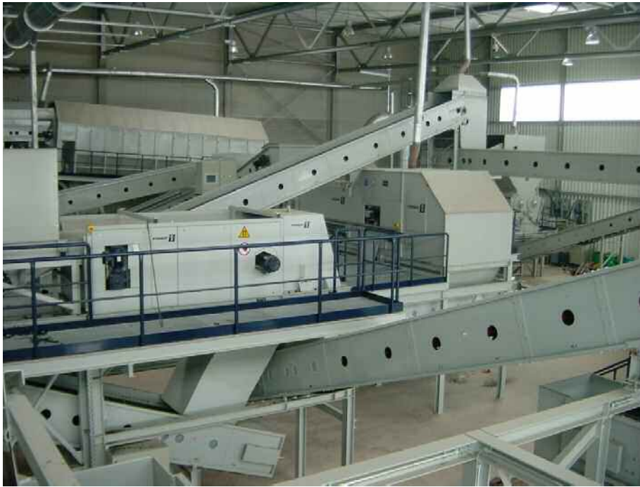
Figure 12: View of an RDF plant with an eddy current separator on the left and an induction sorting system combined with a near-infrared camera on the right side
