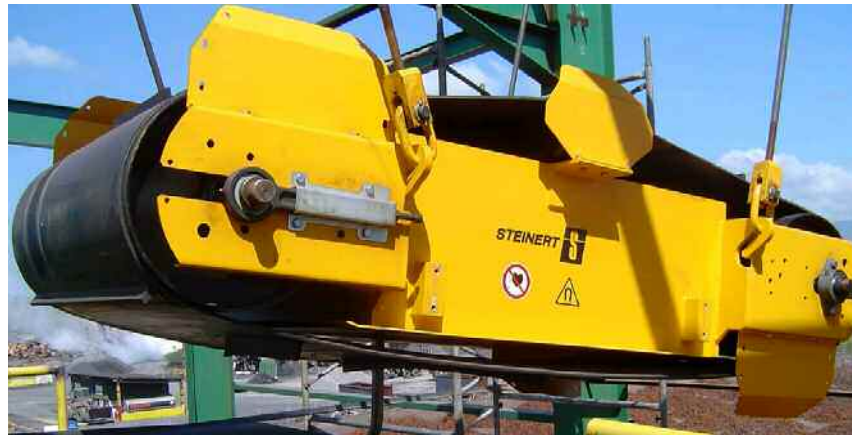
Figure 3: Suspended magnet positioned lengthwise above dropping point
