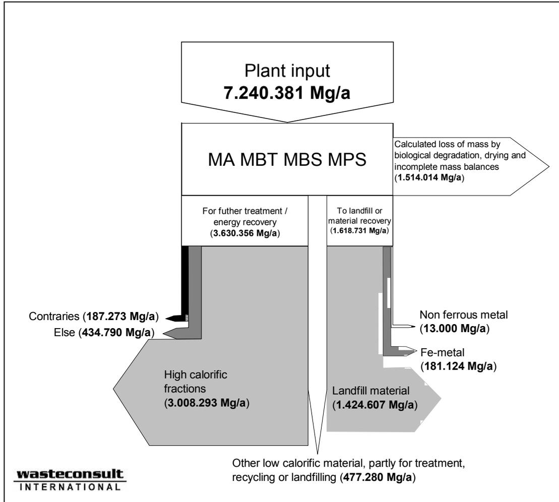
**Figure 3-1 Material flow extrapolated to the overall stock of plants (76\*) in 2006**
