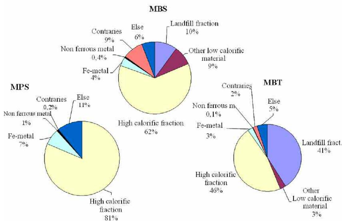
**Figure 3-2 Fractioning of output flow with regard to total output (without loss due to degradation and drying) of the different plant concepts**
