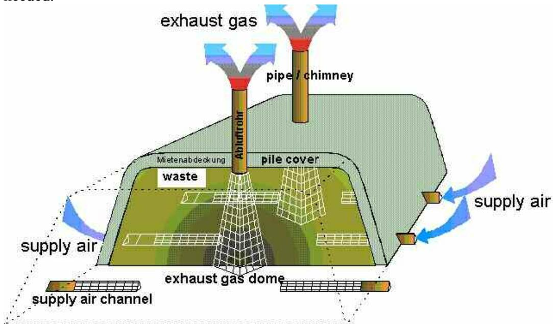
Figure 1 Dome aeration windrow (modified from Brummack et al., 2004)
